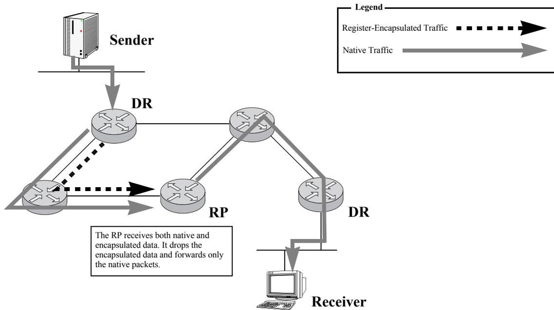
A register-stop packet is sent back to the sender's DR to prevent the DR from unnecessarily encapsulating the packets. Once the register-encapsulated packets are discontinued, the packets are flowing natively from the sender to the RP—along the source-specific tree to the RP and, from there, along the shared tree to all receivers.
