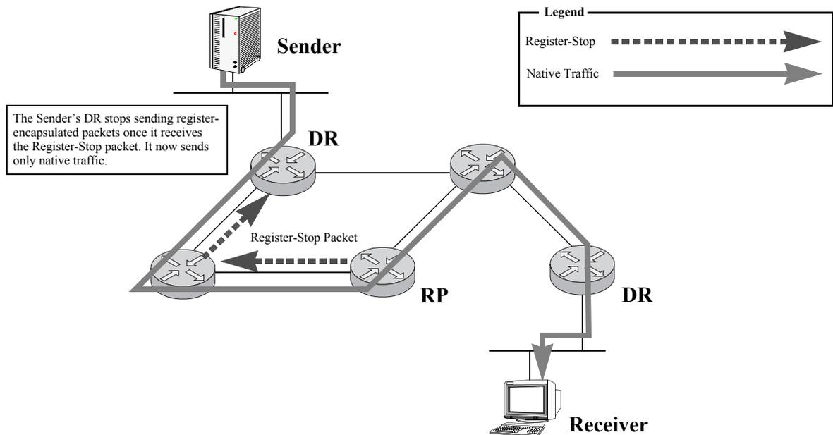
Because packets are still forwarded along the shared tree from the RP to all of the receivers, this does not constitute a true Shortest Path Tree (SPT). For many receivers, the route via the RP may involve a significant detour when compared with the shortest path from the source to the receivers.
