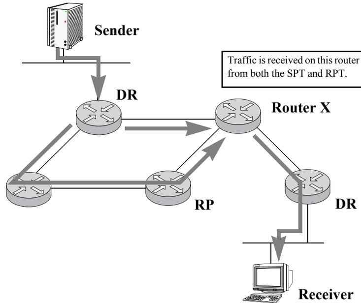
An (S, G, RPT) Prune message is sent toward the RP. As a result, traffic destined for this group from this particular source will no longer be forwarded along the RPT. The RP will still receive traffic from the Source. If there are no other routers wishing to receive data from the source, the RP will send an (S, G) Prune message toward the source to stop this unrequested traffic.
