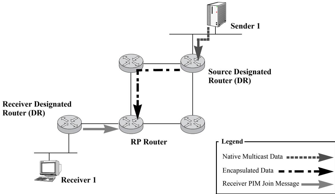
Once the distribution tree for group G is learned at the RP, the encapsulated data being sent from the source DR is now unencapsulated at the RP and forwarded natively to the Receiver.
