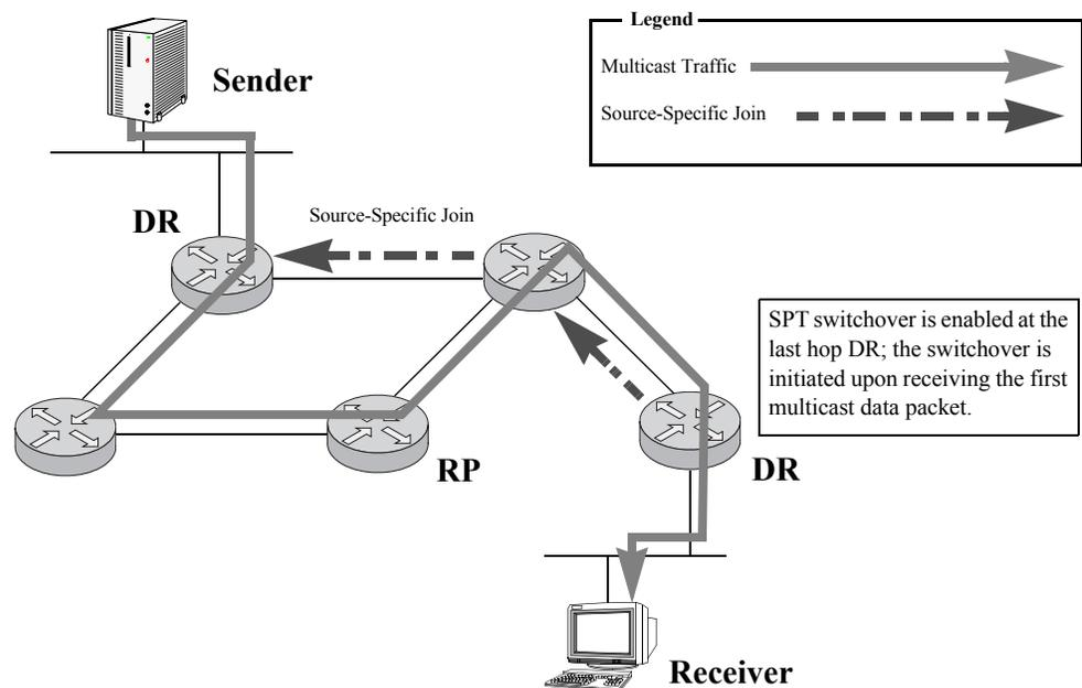
Once the Sender's DR receives the (S,G) Join message, it sends the multicast packets natively along the Shortest Path Tree. At this point, Router X (the router shown between the Sender's DR and the Receiver's DR) will be receiving two copies of the multicast data—one from the SPT, and one from the RPT. This router drops the packets arriving via the RP tree and forwards only those packets arriving via the SPT.
